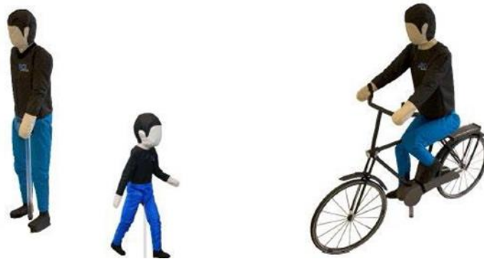
Figure 6: Euro NCAP Pedestrian and Bicyclist and bike Targets (EPTa, EPTc and EBT)
