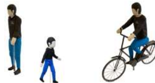
Figure 6 : Euro NCAP Pedestrian and Bicyclist and bike Targets (EPTa, EPTc and EBT)
