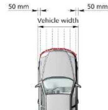
Figure 3 : Virtual profiled line around vehicle front end
