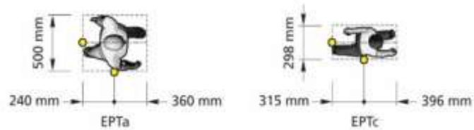
Figure 3-4 : Virtual box dimensions around EPTa and EPTc
