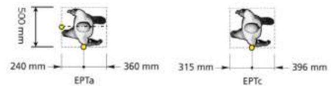
Figure 4 : Virtual box dimensions around EPTa and EPTc
