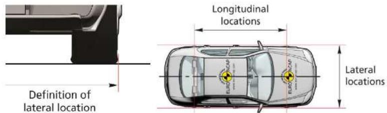
Figure 6-5 : Vehicle dimensional measurements
