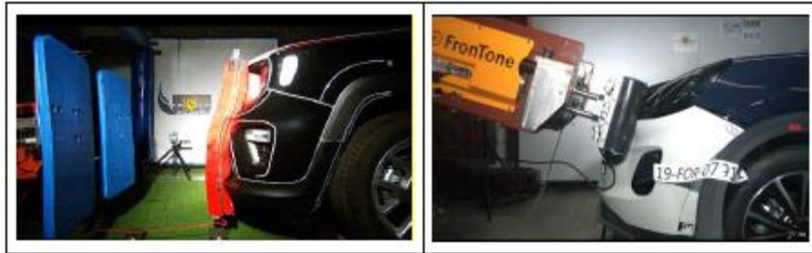
Examples showing correct (left) and incorrect (right) test number location, logo display material, background location
