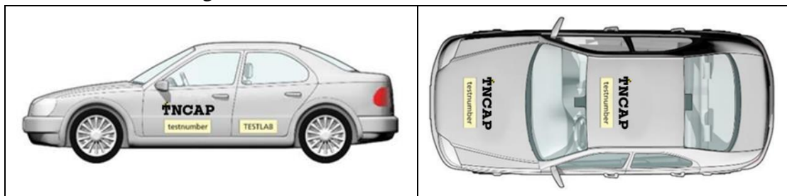
Figure 1: Standardized labels on L/R side, the bonnet and roof area of the test vehicle
