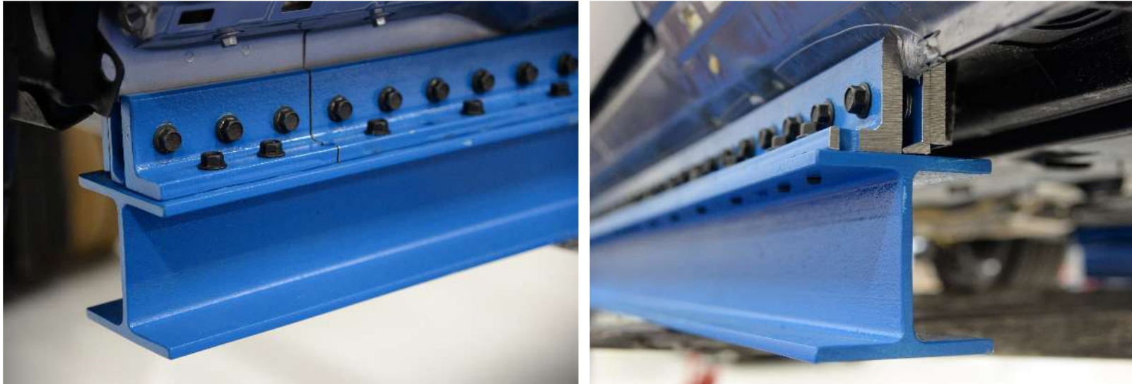
Figure 1: Rocker Panel Support System Attached to the Vehicle
