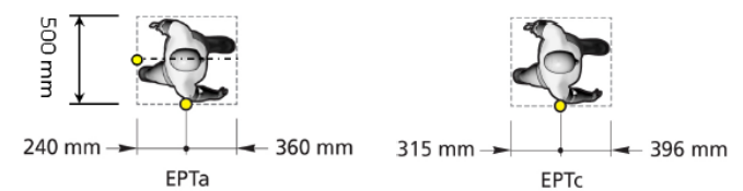
Figure 4 : Virtual box dimensions around EPTa and EPTc
