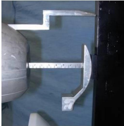
Figure 21 HRMD with backset and height calibration
