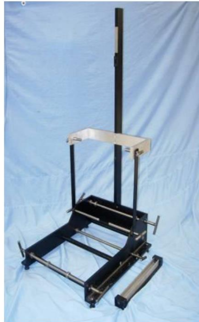
Figure 14 The HPM/HRMD calibration jig (GLORIA)
