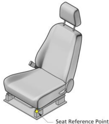
Figure 1: Definition of the Seat reference point
