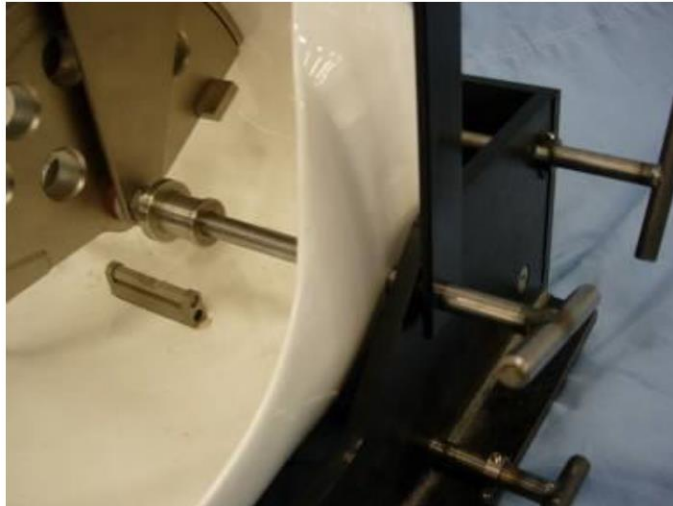
Figure 16 H-point locator bars installed through vertical support rods, jig side and HPM H-point location
