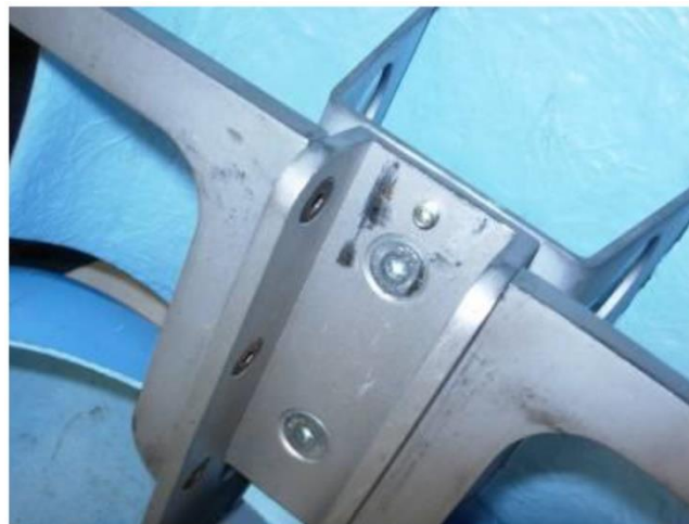
Figure 15 The modified weight hanger assembly
