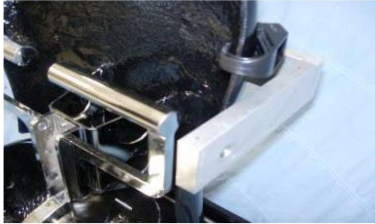
Figure 17 HPM back pan held by support strap
