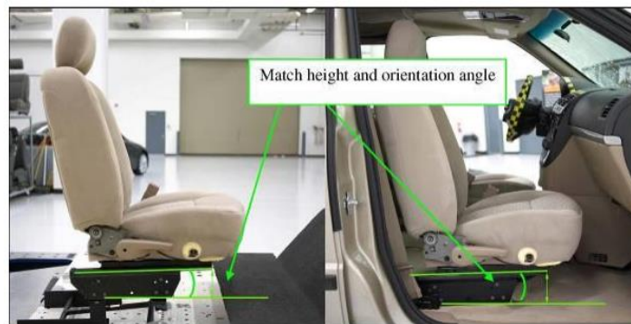
Figure 4 Attachment of seat to test sled
