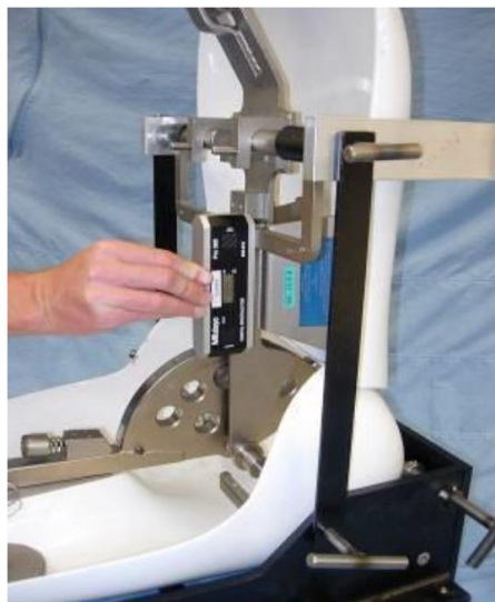
Figure 22 Measurement being taken of the torso angle at the weight hanger trunk by a digital inclinometer
