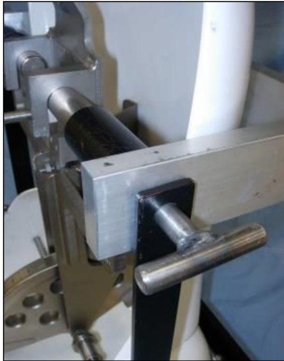
Figure 18 Weight hanger support pins inserted through weight hanger guide bars 3.5.11.8 Calibration of the H-PM Unit
