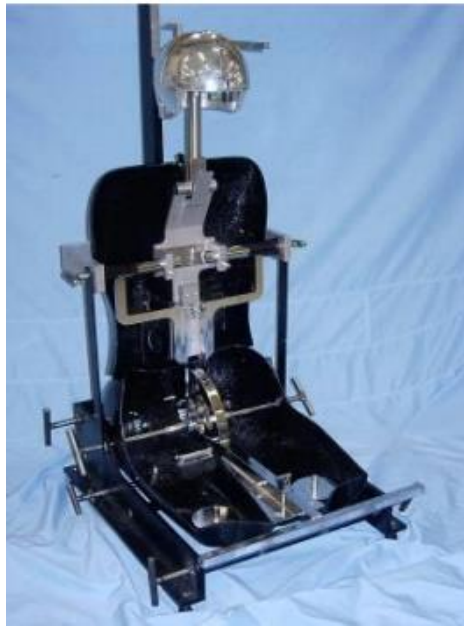
Figure 20: H-PM in calibration jig with H-point to arm supports
