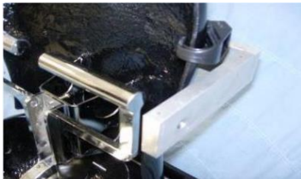
Figure 21: H-PM back pan held by retaining strap.
