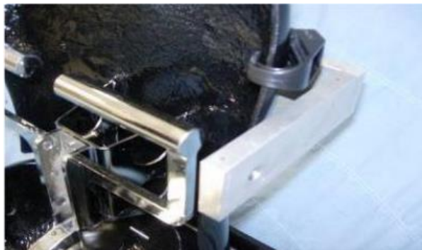
Figure 17: H-PM back pan held by retaining strap.
