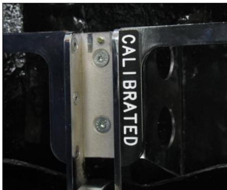
Figure 23: Calibrated Torso angle measurement surface block attached to trunk of weight hanger arm.
